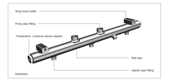
P+P's H<sub>2</sub> rails are used in direct injection processes to ensure the safe supply of hydrogen with an even distribution to the injectors while reducing pressure pulsations.
